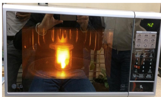
Fig. 3. Snapshot of the oven during the reduction process of GO3. Note the ionization of the atmosphere as GO3 becomes conductive due to reduction.
