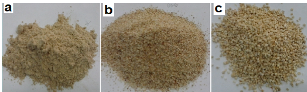
Fig. 2. Aspect of the particles inserted in the composite: (a) fine particle (b) medium particle (c) large particle.
