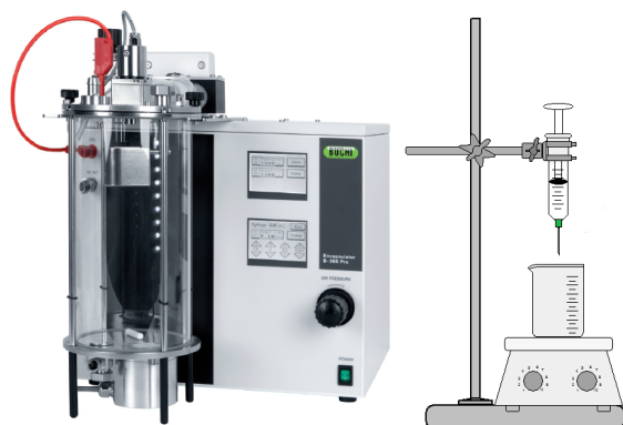
Fig. 8. Buchi® equipment for microencapsulation by extrusion and handmade microcapsule extrusion.
