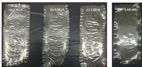
Fig. 1. Representative images of films based on linseed mucilage (LM) at concentrations of (a) 2.0%, (b) 2.5%, (c) 3.0%, and (d) 3.0% with H. virginiana (Hv) extract, forming an antimicrobial film.
