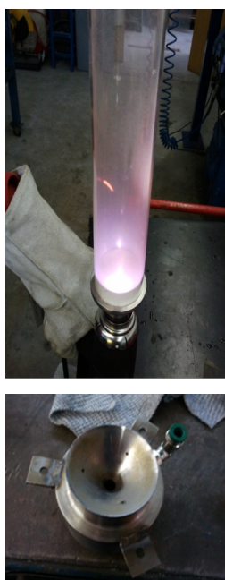
Fig 2. Photographs of the Plasma SFB in operation (top) and the flow distributor cone with slanted jet orifices and a central hole for the plasma torch (see video in supplementary data).
