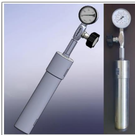
Figure 1. Home-built reactor for oleic acid esterification reactions.
