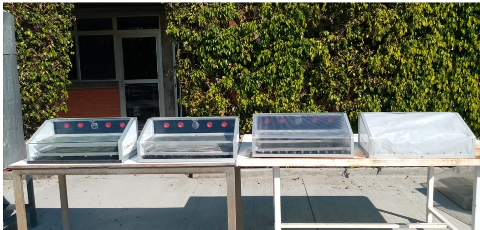
Fig. 1. Drybox Mini2 with different drying covers (From right to left: Polyethylene, polycarbonate, acrylic, and glass).
