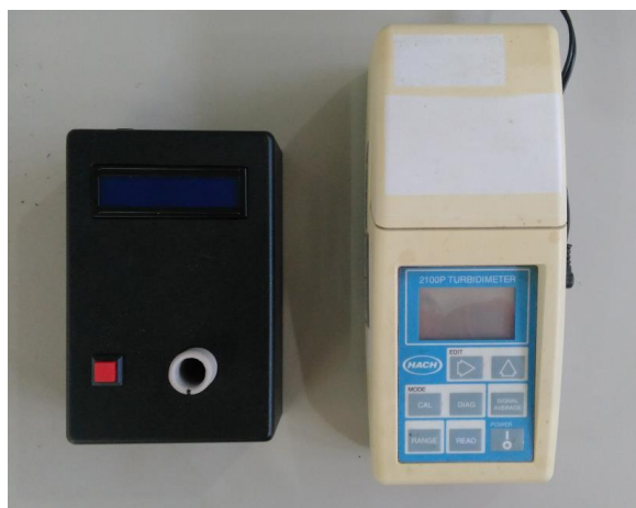
Fig. 6. Turbidimeter developed (left) and 2100P turbidimeter (right).
