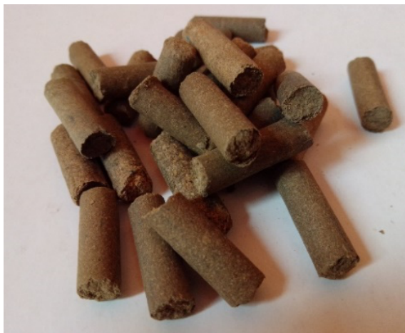
Figure 3. Fuel pellets obtained with 15% of moisture content, 25% of rice husk and 75% of bean straws.
