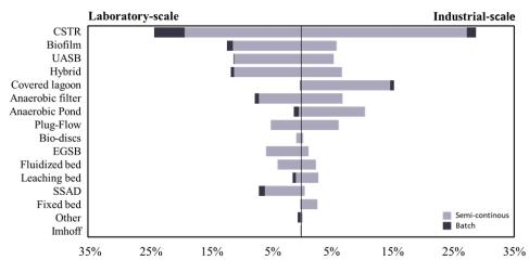
CSTR: Continuously stirred reactor; UASB: Upflow anaerobic sludge blanket; EGSB: Expanded granular sludge bed; SSAD: Solid state anaerobic digester.
