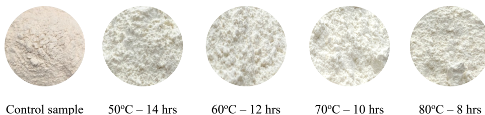
Figure 6. WFSP powder samples were blanched and dried at different temperatures and times compared to the control sample.
