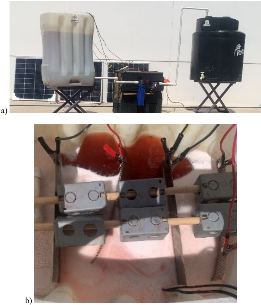
Fig. 2. Electrolytic reactor prototype: a) Side view, b) Internal view of the reactor.
