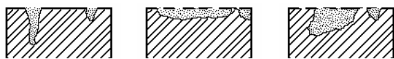
Fig. 2. Schematic presentation of cross-sections of non uniform (localized) forms of corrosion attacks.
