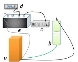
Fig. 2. Electric Field system with variable voltage, (a) source of high voltage, from 5 to 80 kV, (b) treatment chamber with stainless steel circular electrodes, (c) generator and modulator of frequency from 5 to 5,000,000 Hz, (d) oscilloscope, (e) control unit for voltage.
