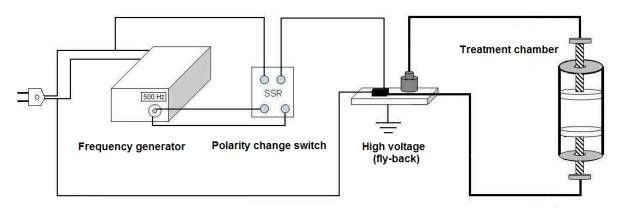
Fig. 1. Diagram of the Electric Field system with constant voltage, (18 kV).
