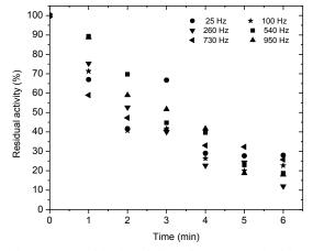
Fig. 4. Residual activity of polyphenoloxidase extracted from avocado as a function of the time of EF treatment at 10 kV/cm.
