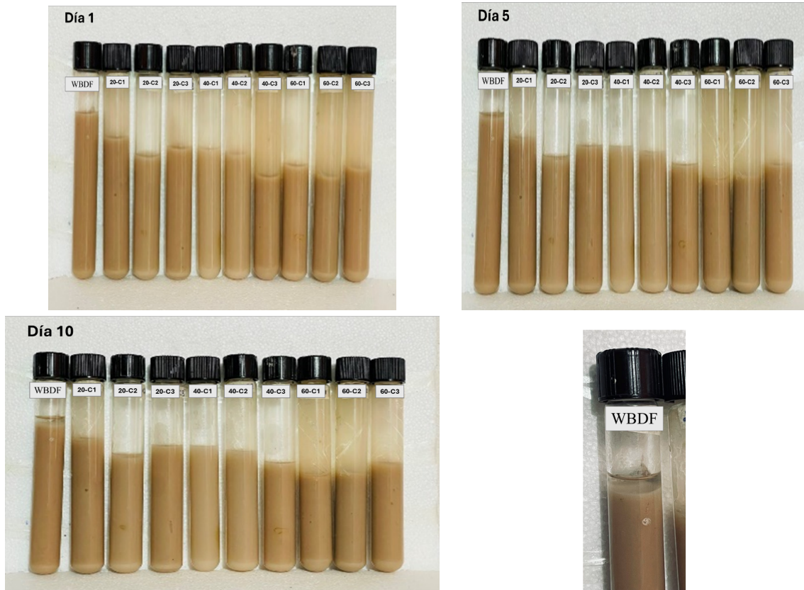
Figure 14. Samples of ZnO-NPs-based drilling fluid formulations and WBDF: a) day 1, b) day 5, c) day 10 and d) separation of water in the WBDF.
