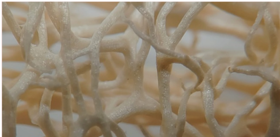
Figure 1. Luffa cords under the light microscope at 32x magnification.
