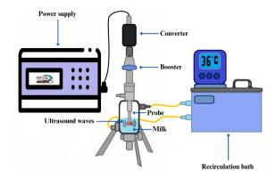
Figure 1. Equipment for thermoultrasonication.
