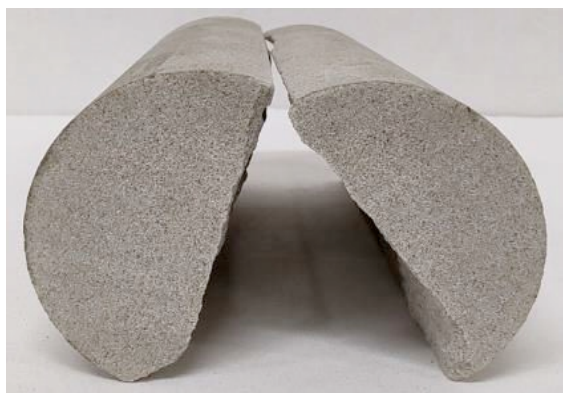
Figure 3. Fractured sandstone rock core before the fluid control test.
