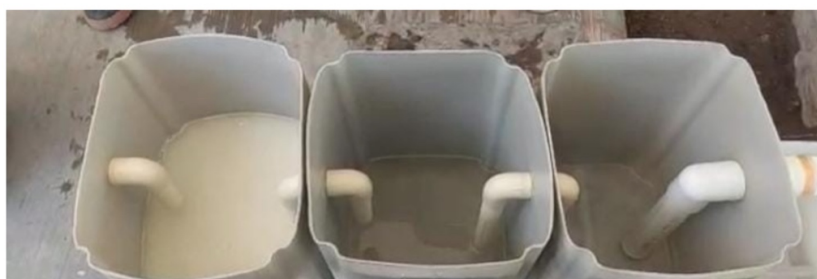
Figure 4. Subsurface horizontal flow wetland diagram (a) with the incorporation of the grease trap (b) for the pre-treatment of acid whey.
